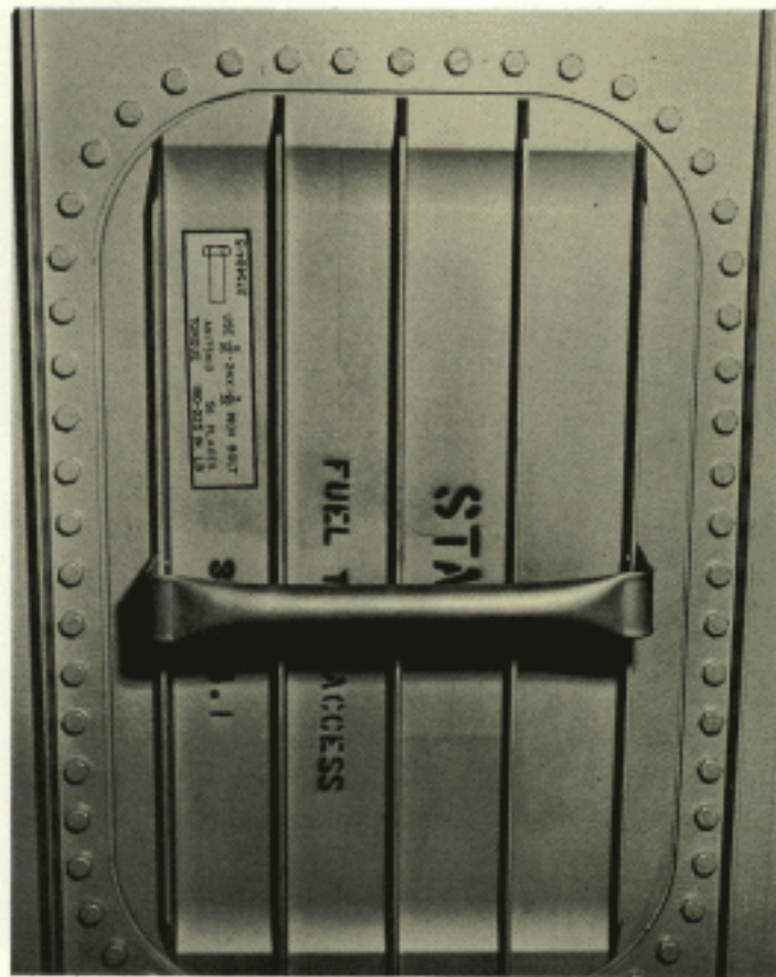
Decal on access panel shows bolt requirements. Here dome nuts are fastened to the removable panel.
